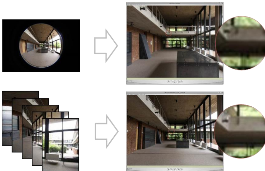
FIGURE IV.A.4 The quality of the panoramic image varies according to the lens used for shooting (a) Sigma 4.5 mm fisheye lens (b) Canon 17-85mm conventional lens
