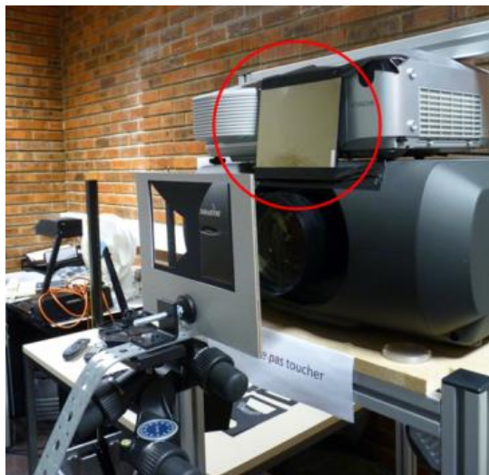
FIGURE IV.A.16 The tinted glass placed in front of the second projector to reduce displayable luminances
