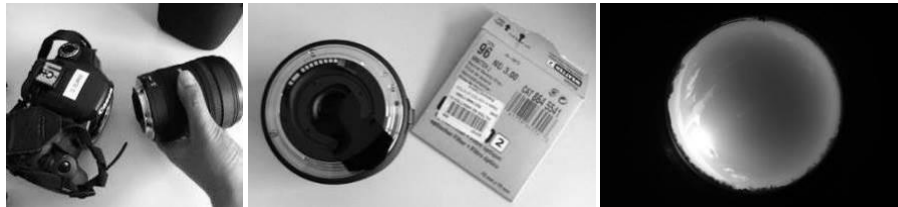
FIGURE V.A.3 Location of the neutral density filter and resulting circular picture
